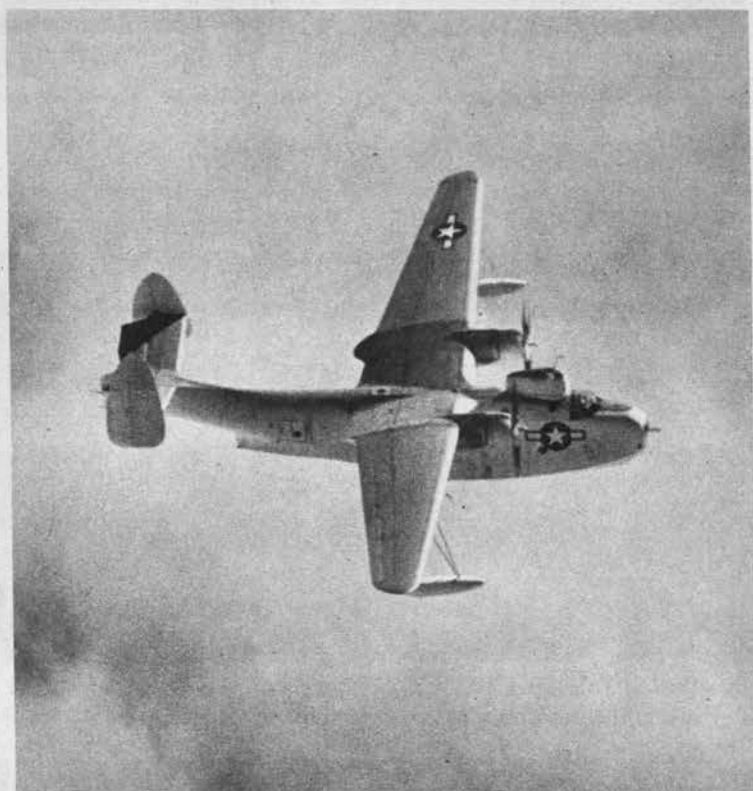
PBM has deep fuselage, gull wing mounting two engines. Fingernail fins, rudders slant; are outboard of the tailplane which has dihedral.
